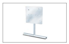
**XP-1-...** predrilled stainless steel (type 304) mounting bracket designed for mounting Thermon junction boxes and thermostats directly to the pipework. The bracket is easily secured to the pipe using B-4, B-10 or B-21 attachment bands. The XP-1 utilises a 110-mm standoff.
