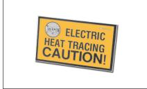
**CL...**vinyl-based peel-and-stick caution labels are intended for direct exposure to industrial environments. Electrically heated pipelines and vessels should be clearly identified at frequent intervals along the pipeline or vessel. Caution labels should be placed at 3 to 6-m intervals or as required by code or specification. Additional languages or other texts are available; contact Thermon.
