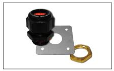
**Insulation Entry Kits (IEK)...** are used for inserting permanent circular and noncircular cables into the insulation. The kit protects and seals the cable while penetrating the insulation cladding.
