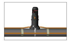
Terminator ZS/ZE...designed to fabricate accessible outside-the-insulation splices or end terminations of Thermon Heating Cables. Electrical connections are made using wire fasteners (for applications requiring terminations to be made with terminal block connections, the Terminator ZP kit may be used).
