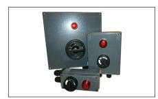
**CS-L-\*-Ex....** Circuit switch with lamp to be used as an in-line isolation switch for single phase, phase-phase and 3-phase heat tracing circuits. Available in 16 A, 25 A and 40 A versions.
